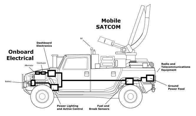
Figure 2 shows an overlay of the necessary "Faraday Cage" constructs at each critical subsystem of the vehicle, with bonding between systems and filters at each POE.
