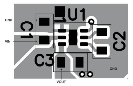
Figure 4. 140-mA, 5-V TPS60150 Charge-pump Layout Example
