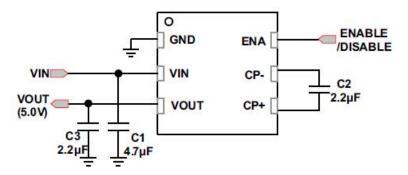
Figure 3. 140-mA, 5-V TPS60150 Charge-pump Circuit
