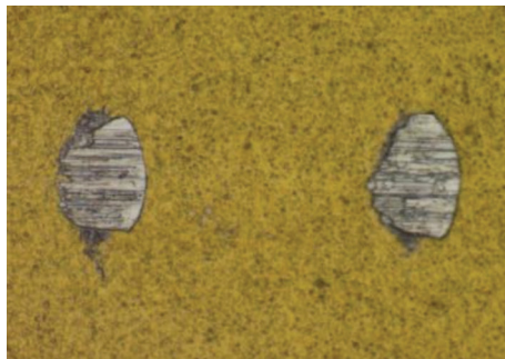
Figure 2. Sheared wire bonds.
