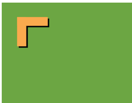
Die placement fiducial on substrate – without die.
