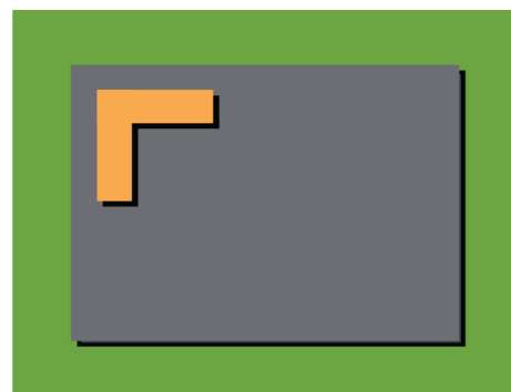
Die placement fiducial covered by die – can be assembled, cannot be measured after.
