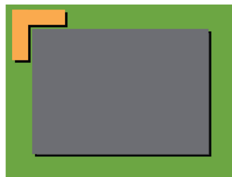
Die placement fiducial outside of die – can be assembled, can be measured after.
