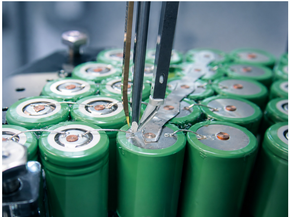
Figure 1. Process tooling – end effector, cutter, and clamp
